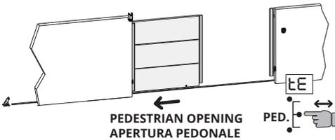
3. Press and release the PEDESTRIAN key. The gate memorizes the pedestrian opening point.
