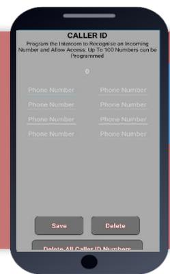
Enter up to 8 numbers per SMS for CallerID & press save to create the text string. (max 250 separate numbers)
