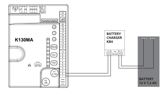
To ensure the gate operation during a power failure, the KB4 kit (battery charger + battery 12V 7.2Ah) can be used to connect to the control unit as shown in the diagram above. **NOTICE: the battery cannot be connected directly to terminals 1-2 of the control unit.**
