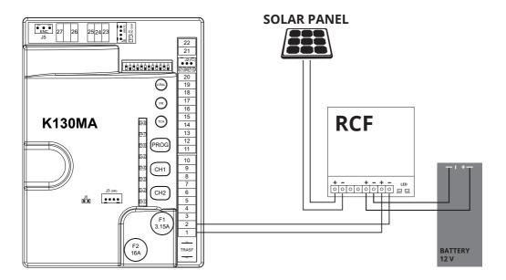
If you do not have the mains voltage to power the gate automation and you want to use renewable energy, you can connect a photovoltaic panel + adjustment board + 12V battery to the automation control unit as shown in the diagram above.
