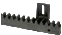
400CN Steel core, fibreglass reinforced, 22x22 nylon rack (Module 4, max 800 kg). Pack of 10 m
