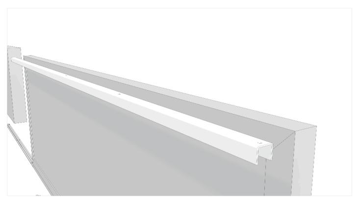
Set the bracket onto the back side of the second leaf.
