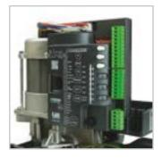
**CONTROL ELECTRONICS** Quick and intuitive programming thanks to signalling LEDs. Two-channel radio receiver built-in the control unit (433,92 MHz, 30 codes to memorize).
